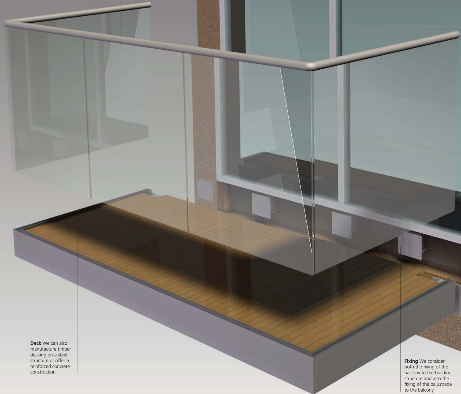
**Deck** We can also manufacture timber decking on a steel structure or offer a reinforced concrete construction
